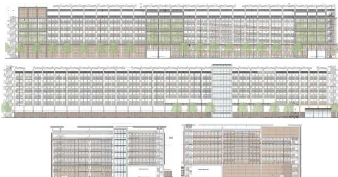
Figure 11. Conceptual North Garage elevations: east (top), west (middle), north (bottom left), and south (bottom right). The building facades are predominantly opaque; glazed areas are located on all levels the elevator towers on the west and north facades.
