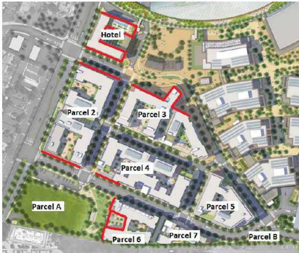
Figure 6. Illustrative site plan showing the proposed residential/mixed-use buildings and associated open space areas. Facades with highest collision risk are delineated in red.
