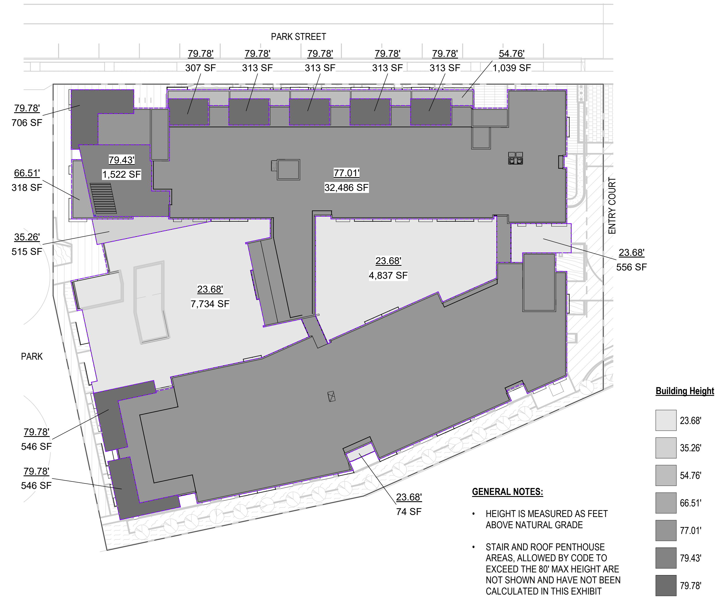
P6 - BUILDING HEIGHT CALCULATION - ROOF 1 1" = 30'-0"
