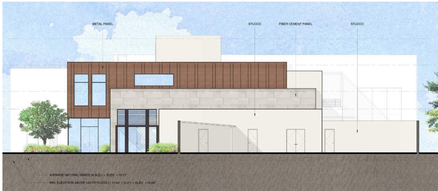
BUILDING ELEVATION - NORTH
