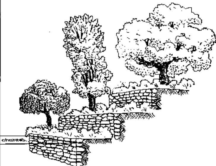
Multiple retaining walls
