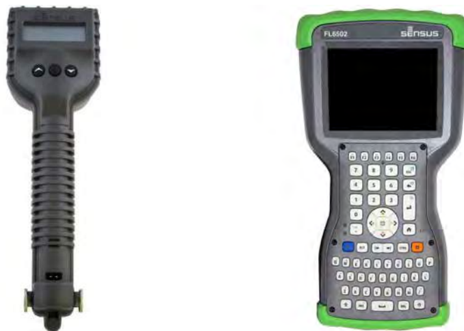
Figure 3. AMR TouchRead Communication Equipment
