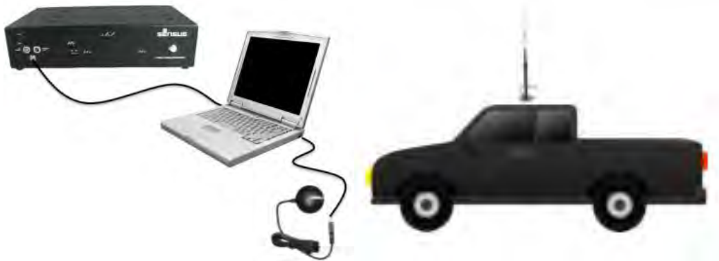
Figure 5. AMR Vehicle Base Station Communication Equipment
