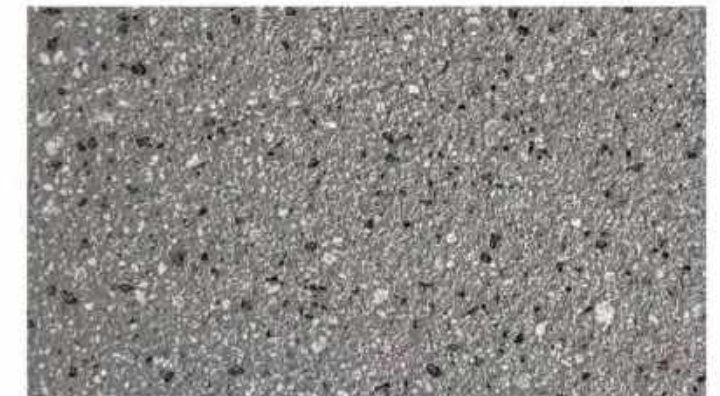
⑦ GFRC, SANDBLASTED, SMOOTH: COLOR TO MATCH DUNN EDWARDS CHARCOAL SKETCH
