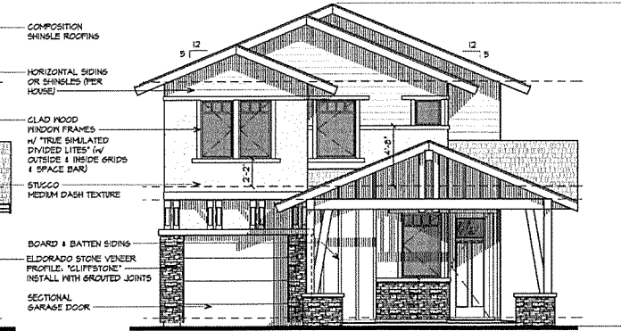
FRONT / SOUTH-EAST ELEVATION
