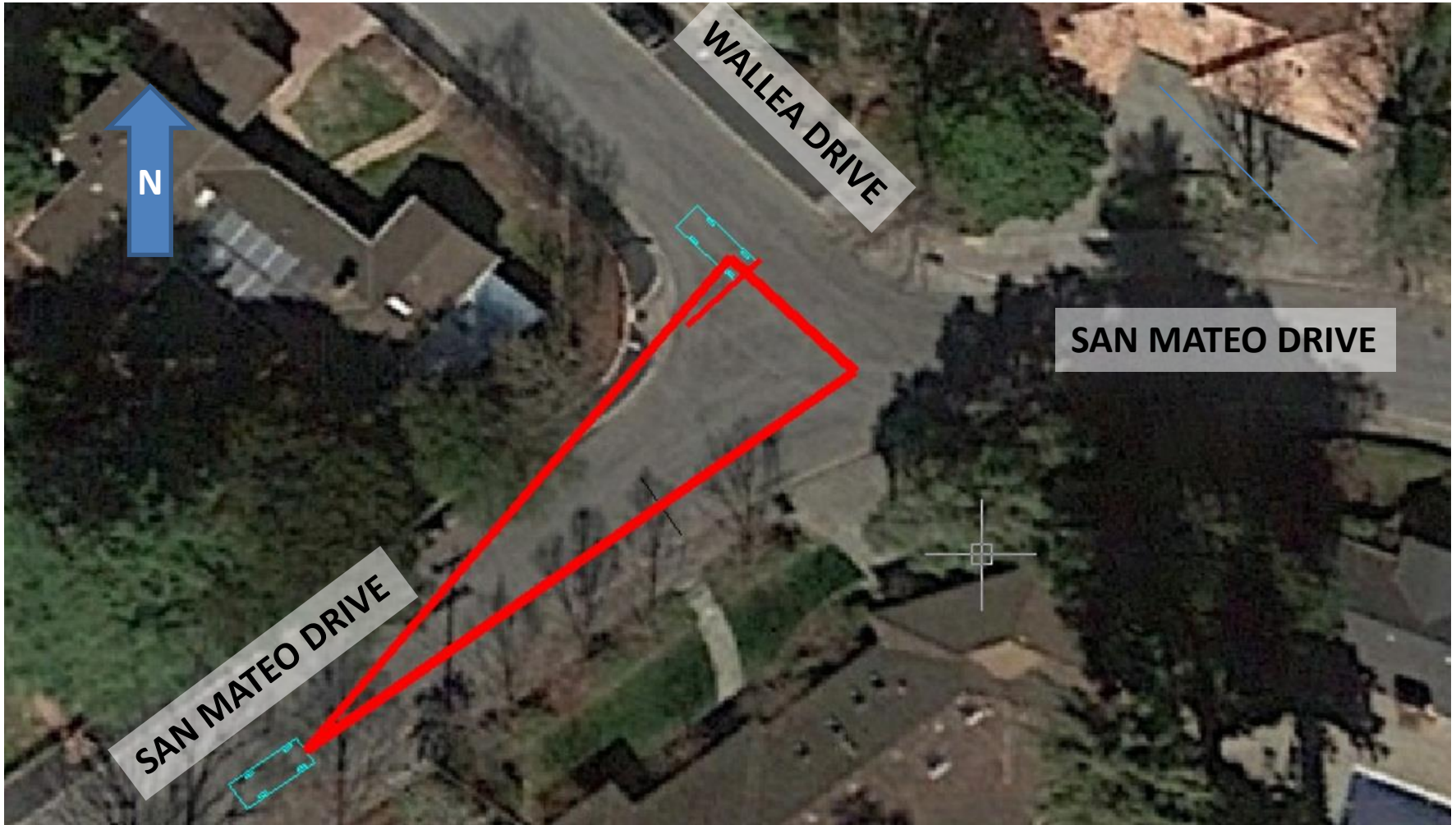
— SIGHT TRIANGLE FOR 25 MPH VEHICLE SPEED ON SAN MATEO DRIVE
