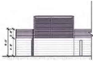
6 TRASH ENCLOSURE - WEST ELEVATION 1/4" = 1'-0"
