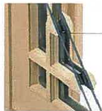
3. Simulated Divided Lite w/ Spacer N.T.S
