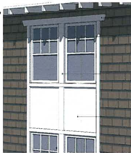
2. Fiber Cement Panel N.T.S
