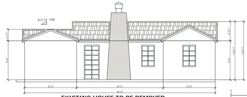
EXISTING HOUSE TO BE REMOVED: SOUTHEAST (REAR) ELEVATION
