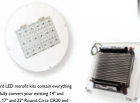
The standard LED retrofit kits contain everything needed to fully convert your existing 14" and 19" Square, 17" and 22" Round, Circo CR20 and Gullwing G13 to any of the available LED wattages and distributions. This includes a reflector pan with LED arrays along with the fully wired pan with attached driver, equipped with quick disconnects.
