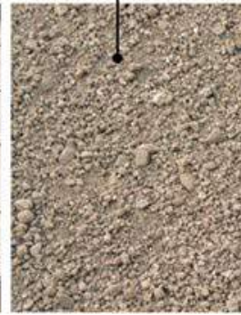
TYPE 6. CRUSHED STONE PAVING
