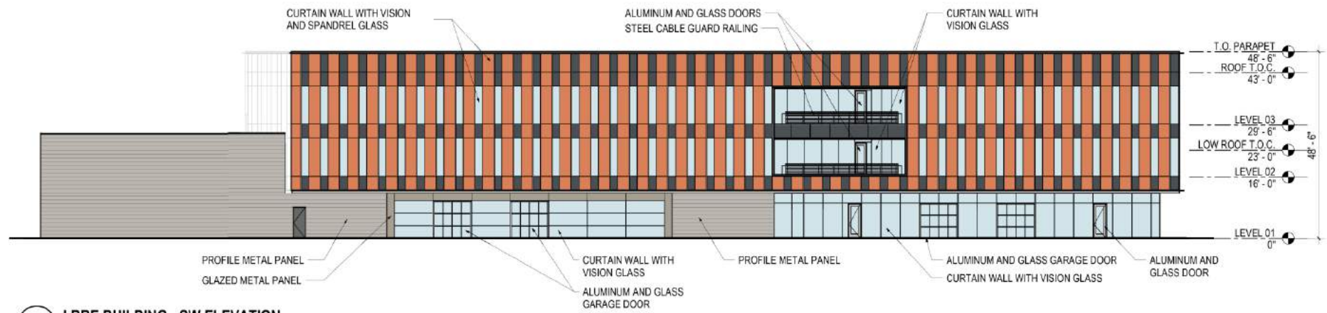
1 A3.1 LBRE BUILDING - SW ELEVATION 1/16" = 1'-0"
