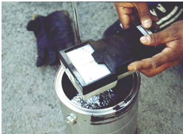
Figure 3-7 Hand Held Viscometer Testing (Analog Model)
