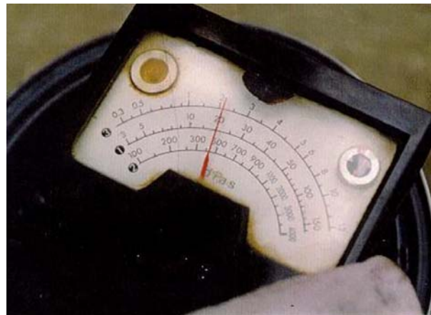
Figure 3-8 Analog Viscometer Reading – Scale No. 1
