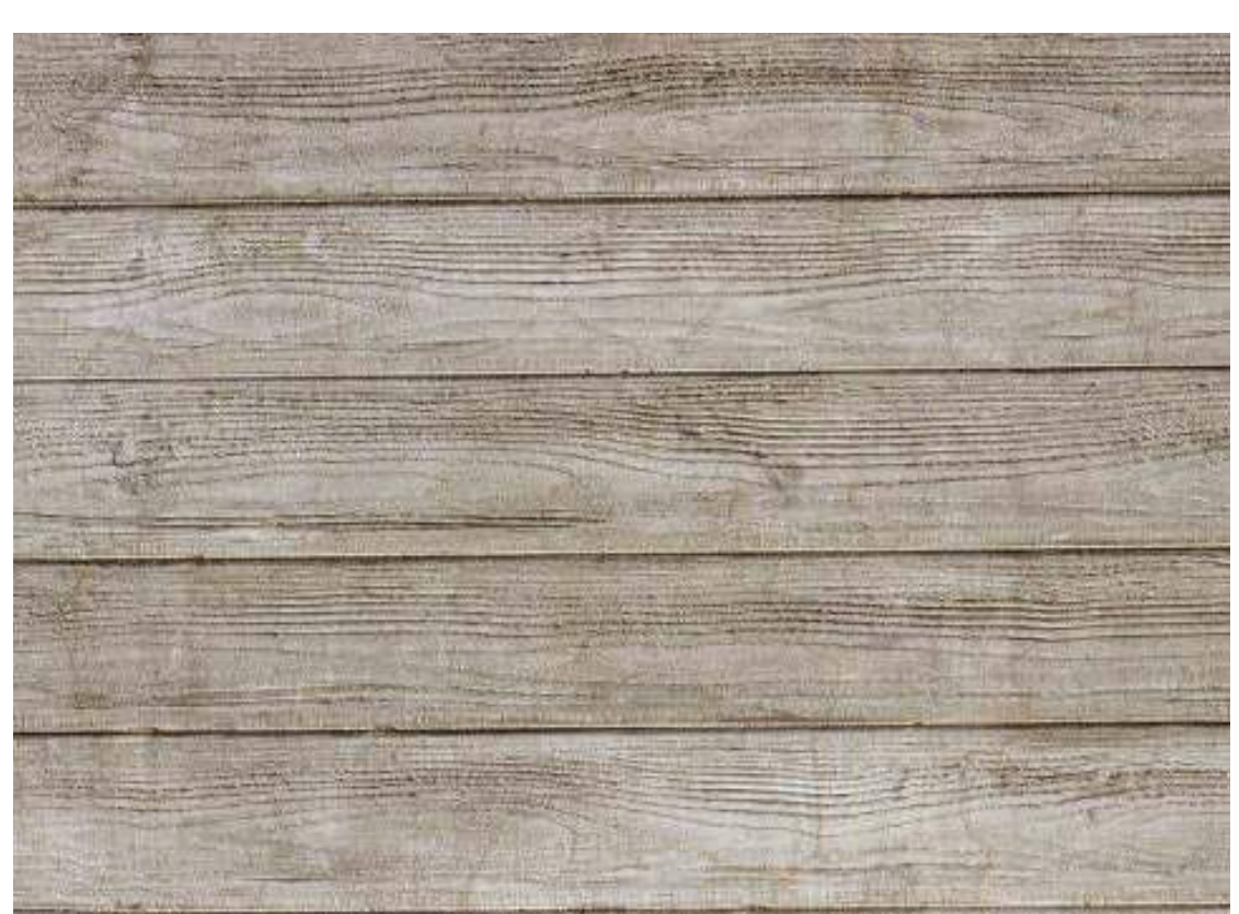
PAVEMENT NODE - STAMPED CONCRETE
