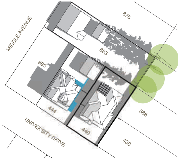
SPRING EQUINOX (MARCH 19) - 9:00 AM SHADOWS CAST ON 444 UNIVERSITY DRIVE = 4.3% OF LOT AREA
