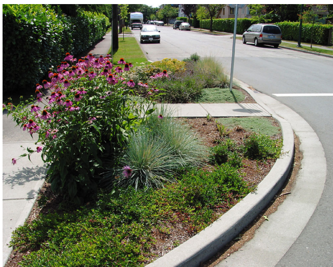
Example of a curb extension with a rain garden.
