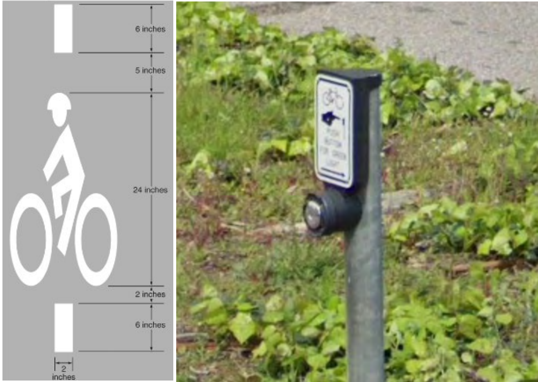
Fig 5-25 Bicycle Detector Pavement Marking and Push Button
