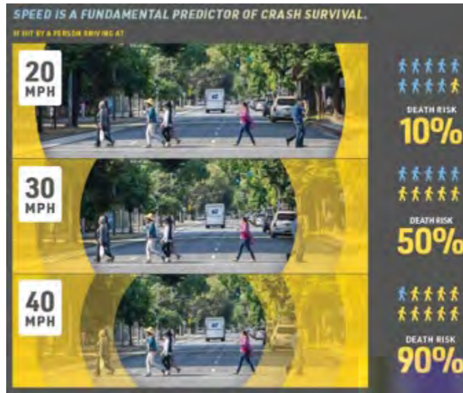
Figure 3 Increasing driver vehicle speed reduces vulnerable road user crash survivability and narrows the driver’s field of vision.
