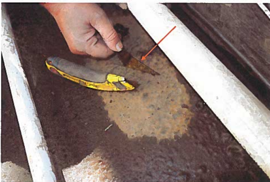
Figure 17 Adhesion pull test was performed on the waterproofing membrane. Adhesion was poor.
