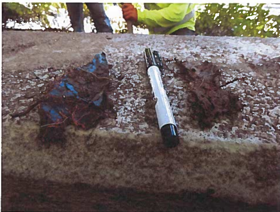
Figure 25 Samples of self-adhering membrane taken from location. Note the extent of root damage caused by the roots penetrating the membrane.
