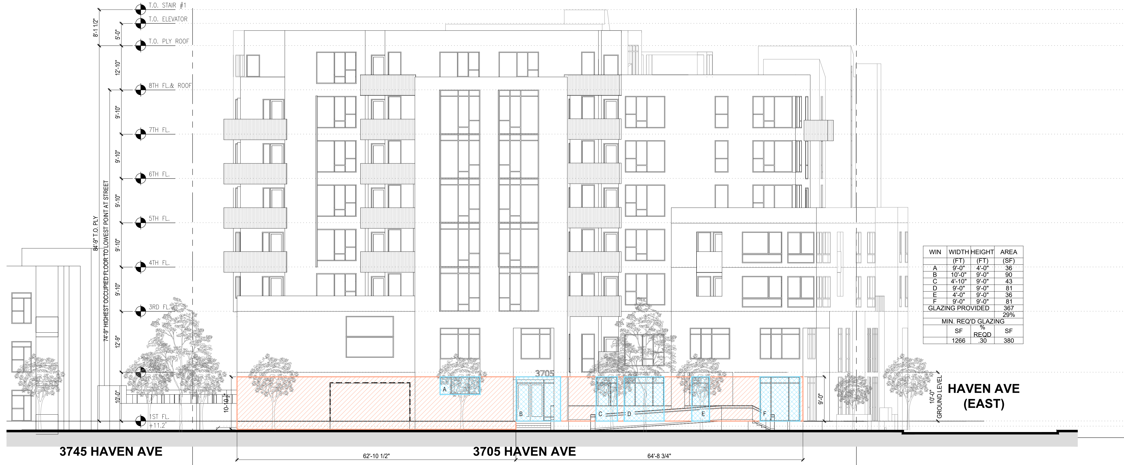
1 ELEVATION : HAVEN STREET SOUTH - GROUND FLOOR TRANSPARENCY 3/32" = 1'-0"
