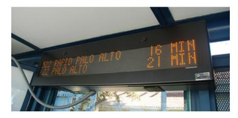
Figure 25 Real Time Arrival Display (VTA Bus Stop)
