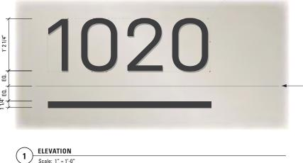
Numbers and accent bar are 1" thick cut out aluminum with paint finish on all exposed surfaces, concealed stud mount flush to metal wall panel, install at equal distances above and below metal panel seam, fabricator to confirm appropriate mounting method to metal wall prior to install
