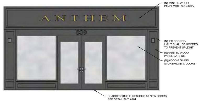
1 PROPOSED SANTA CRUZ AVENUE ELEVATION-RENDERING NO SCALE SEE DIMENSIONS AND NOTES SHEET A500 NOTE: ALL SIGNS ARE UNDER SEPARATE PERMIT.
