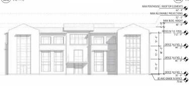
MAX PENTHOUSE / ROOFTOP ELEMENTS MAX ALLOWABLE PROJECTIONS 52' - 0' MECHANICAL SCREEN BEYOND OFFICE N T.O. STEEL 112' - 9" OFFICE N LEVEL 3 OFFICE N LEVEL 2 OFFICE N LEVEL 1 North Office - Front West Elevation
