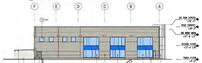
2A BUILDING ELEVATION - EAST - POOL AREA 1/8" = 1'-0"
