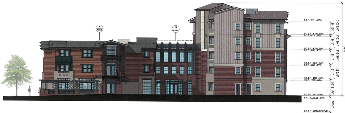
2 BUILDING A - COURTYARD SOUTH ELEVATION 1" = 10'-0"
