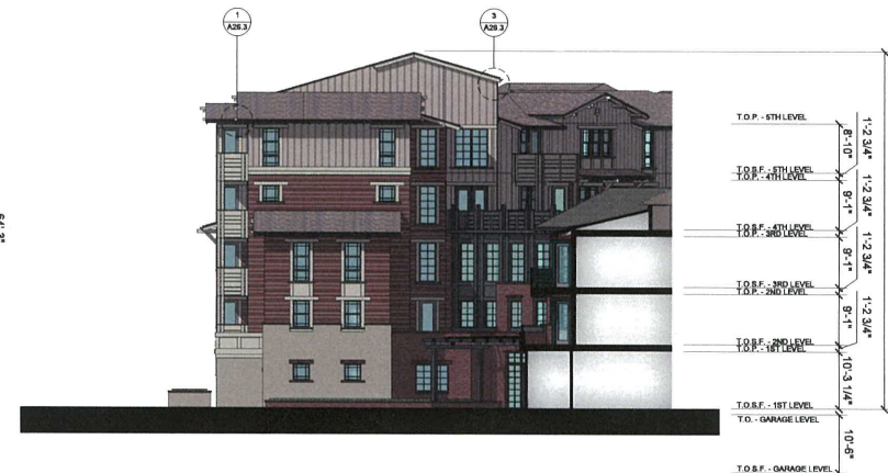
4 BUILDING A - NORTHWEST ELEVATION 1" = 10'-0"
