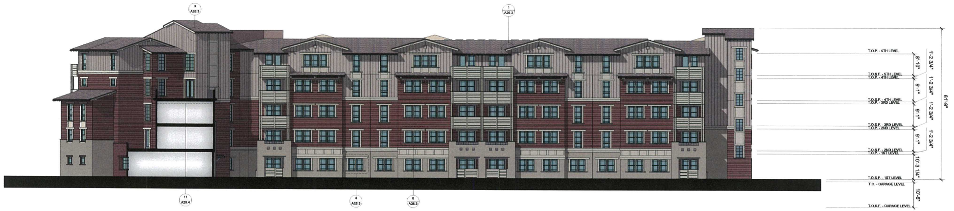
1 BUILDING A - COURTYARD WEST ELEVATION 1" = 10'-0"
