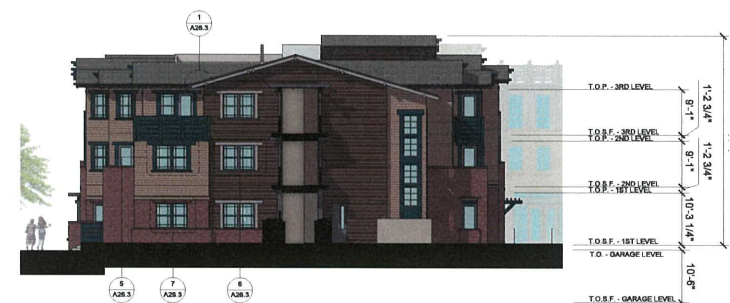
3 BUILDING B - COURTYARD SOUTH ELEVATION 1" = 10'-0"
