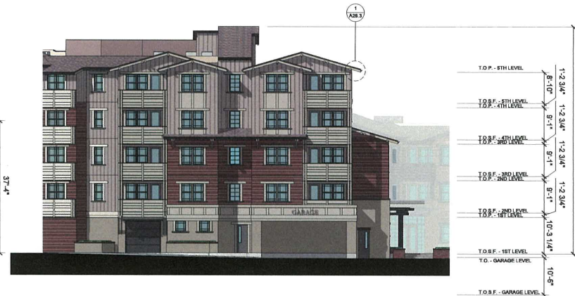
3 BUILDING A - NORTHEAST ELEVATION 1" = 10'-0"
