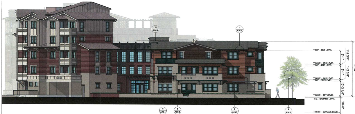
1 BUILDING A - NORTH ELEVATION 1" = 10'-0"
