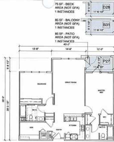
UNIT 7D 2 BED + DEN / 2 BATH GROSS AREA: 1256 SQFT NET AREA: 1186 SQFT 3 INSTANCES
