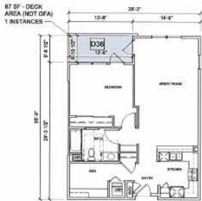
UNIT 1R 1 BED + DEN / 1 BATH GROSS AREA: 900 SQFT NET AREA: 842 SQFT 1 INSTANCES
