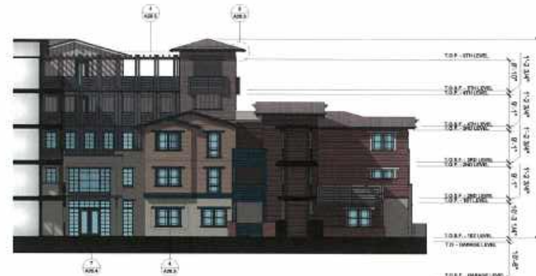
4 BUILDING B - COURTYARD NORTH 2 ELEVATION 1" = 10'-0"
