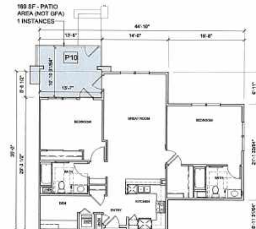
UNIT 7E 2 BED + DEN / 2 BATH GROSS AREA: 1256 SQFT NET AREA: 1180 SQFT 1 INSTANCES
