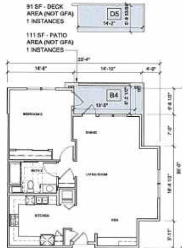
UNIT 10A 1 BED + DEN / 1 BATH GROSS AREA: 996 SQFT NET AREA: 931 SQFT 2 INSTANCES
