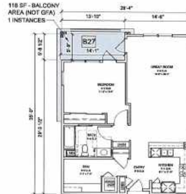
UNIT 1K 1 BED + DEN / 1 BATH GROSS AREA: 904 SQFT NET AREA: 842 SQFT 1 INSTANCES
