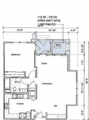
UNIT 10B 1 BED + DEN / 1 BATH GROSS AREA: 993 SQFT NET AREA: 930 SQFT 1 INSTANCES
