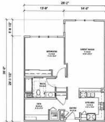
UNIT 1L 1 BED + DEN / 1 BATH GROSS AREA: 899 SQFT NET AREA: 842 SQFT 2 INSTANCES
