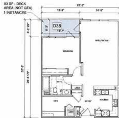
UNIT 1Q 1 BED + DEN / 1 BATH GROSS AREA: 911 SQFT NET AREA: 849 SQFT 1 INSTANCES
