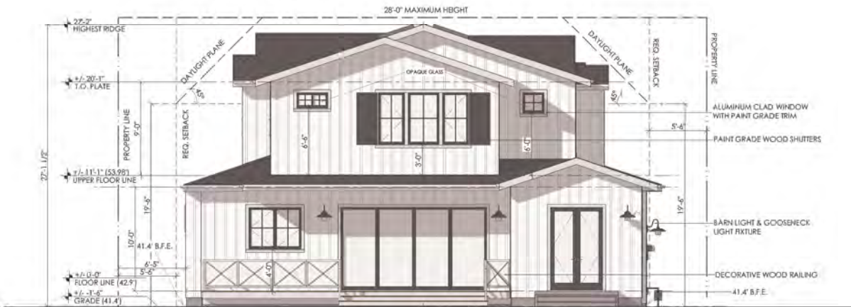
E2 EAST ELEVATION REAR YARD VIEW
