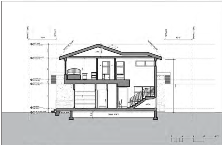
1 BUILDING CROSS SECTION 3/16"=1'-0"
