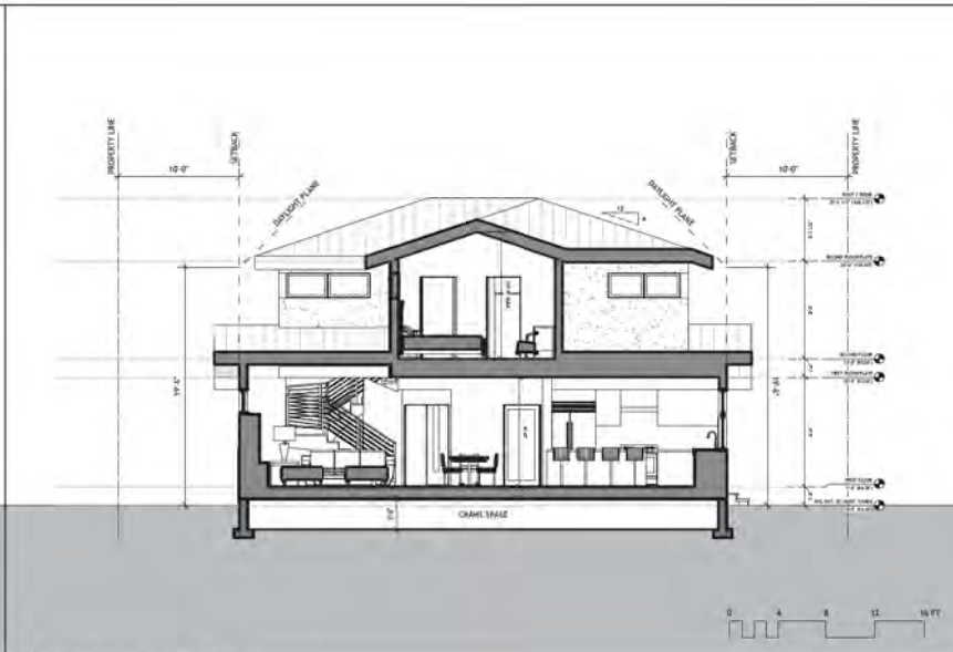
2 BUILDING CROSS SECTION 3/16"=1'-0"
