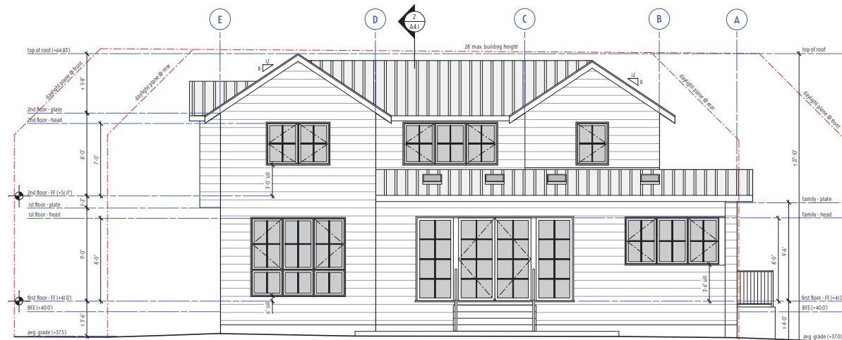
2 east (rear) elevation scale: 1/4" = 1'-0"
