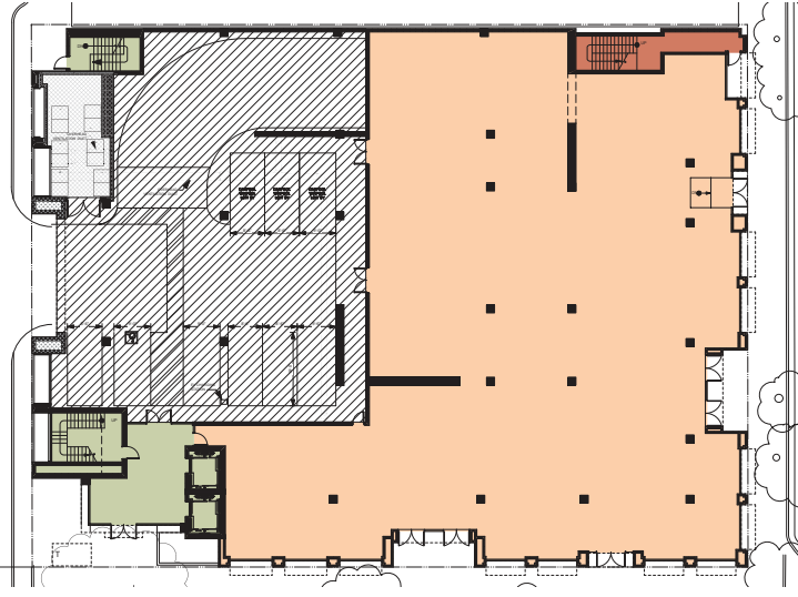
FIRST FLOOR AREA 2 SCALE: 1/16" = 1'-0" Legend: - Hatched area: "M.P.M.C. SECTION 16.04.325 (C) EXCLUSION FOR COVERED PARKING" - Dotted area: "M.P.M.C. SECTION 16.04.325 (C) EXCLUSION FOR TRASH AND RECYCLING" - Stippled area: "M.P.M.C. SECTION 16.04.325 (C) 3% EXCLUSION FOR AREA WITH NO A/C & WINDOWS"
