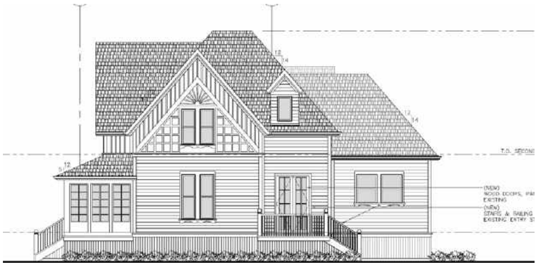
2 SOUTH ELEVATION SCALE: 1/4" = 1'-0"
