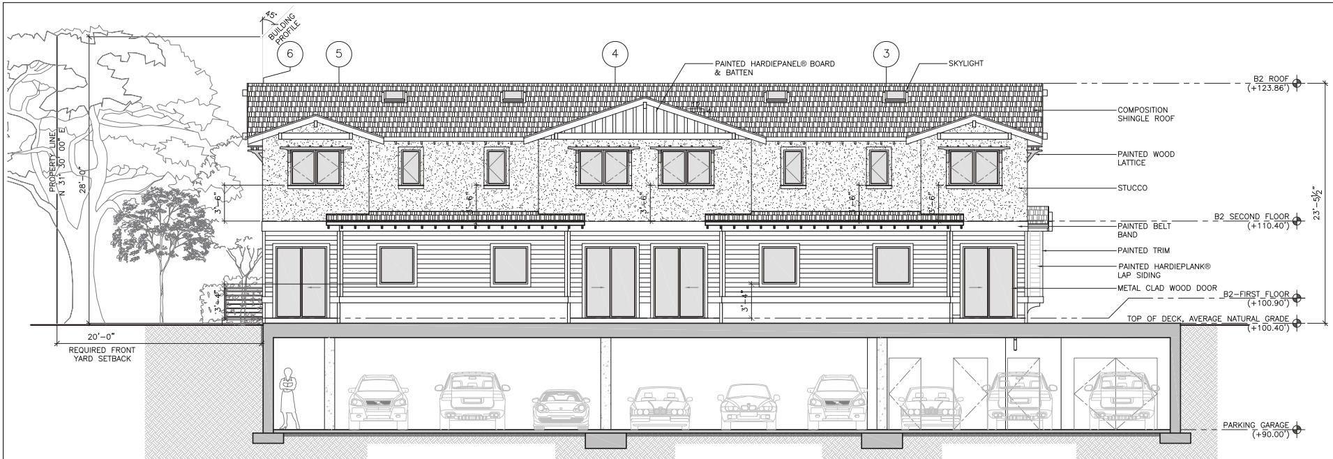
2 SOUTH ELEVATION SCALE: 1/4" = 1'-0"
