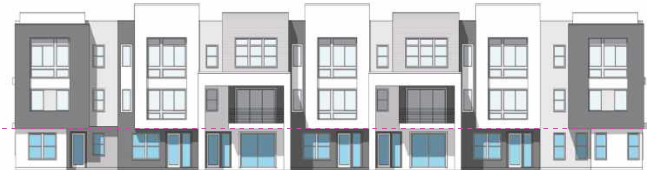
Typical Glazing at Front Elevation
