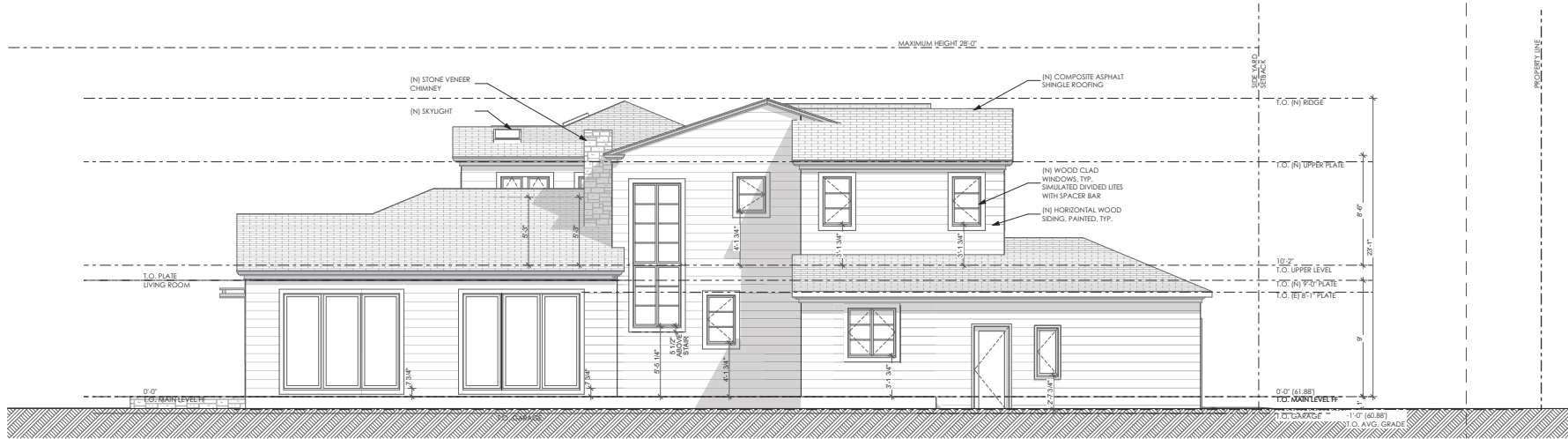
1 A3.3 NORTH (SIDE) ELEVATION - PROPOSED SCALE: 1/4" = 1'-0"
