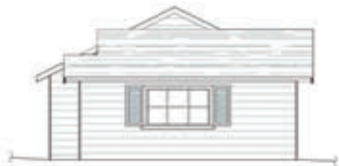
4 cottage - north elevation scale 1/4" = 1'-0"
