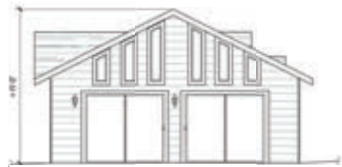
2 cottage - south elevation scale 1/4" = 1'-0"
