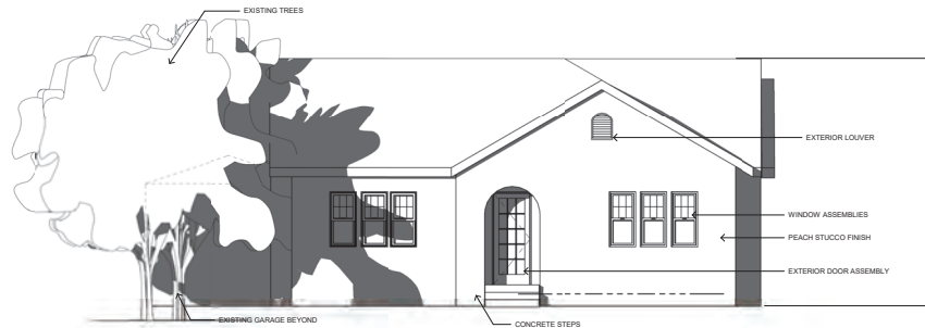
EXISTING - EAST ELEVATION - FRONT 1/4" = 1'-0"
