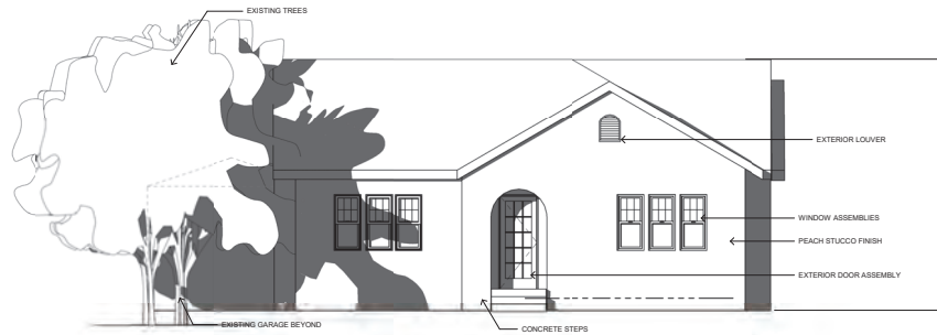
EXISTING - EAST ELEVATION - FRONT 1/4" = 1'-0"
