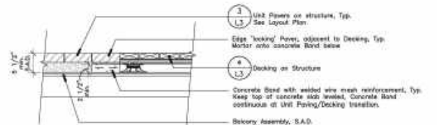
7 Unit Paving to Decking Condition
