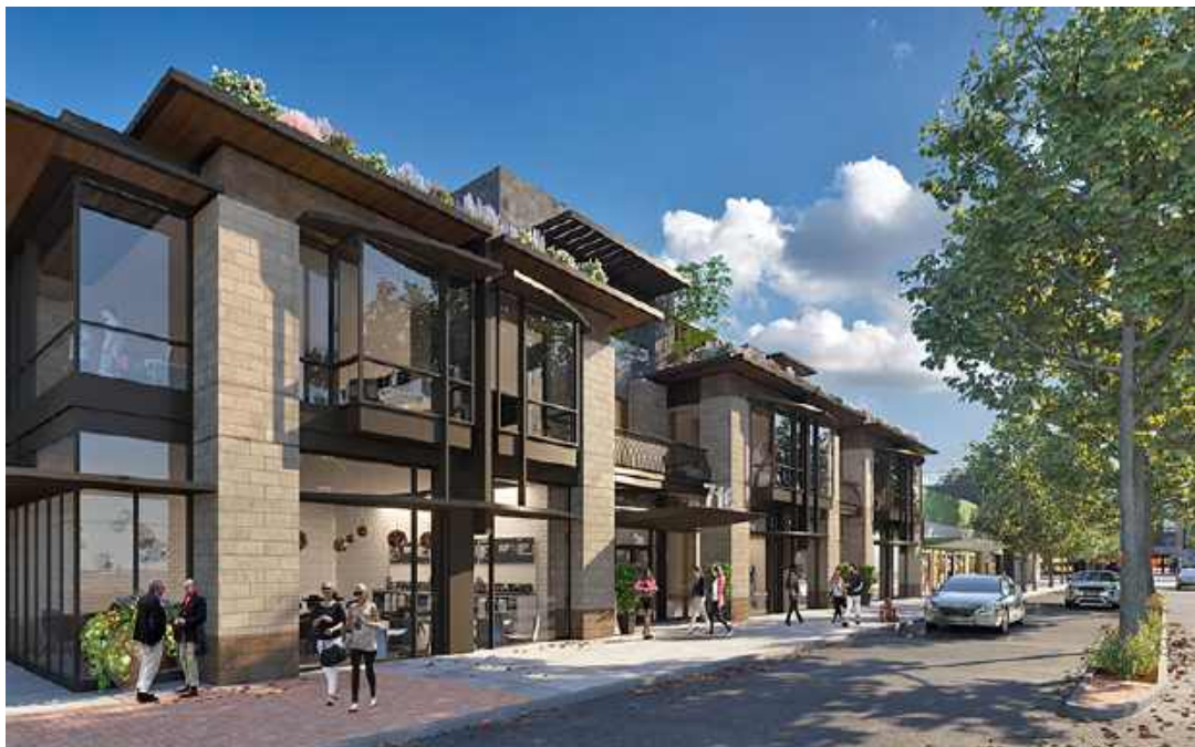
The building is scaled to fit in with the existing context. A strong horizontal cap at the top of the second floor makes the overall building mass appear as two story. Due to sight lines, the third floor is not readily perceived by the public.
