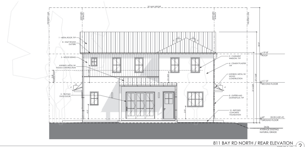
811 BAY RD NORTH / REAR ELEVATION SCALE 1/4" = 1'-0" ②
