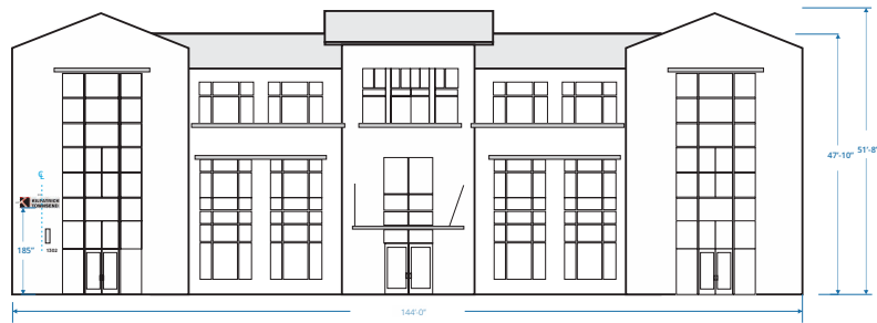
2 NORTH OFFICE BUILDING - EAST ELEVATION scale: 1/12"=1'-0"
