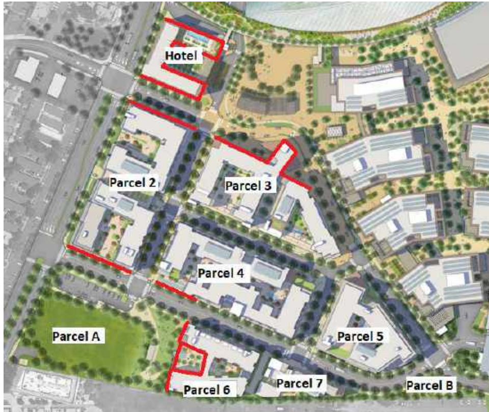
Figure 6. Illustrative site plan showing the proposed residential/mixed-use buildings and associated open space areas. Facades with relatively highest collision risk are delineated in red.
