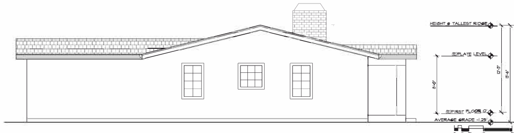
4 EXISTING HOUSE LEFT SIDE ELEVATION (WEST)
