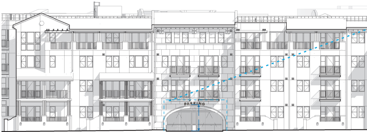
RESIDENTIAL BUILDING - EAST ELEVATION scale: 1/16" = 1'-0"
