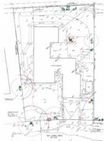
Location of existing house, trees requested for removal protected trees and their Tree Protection Zones
