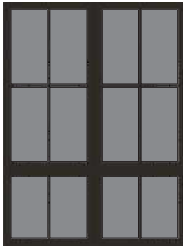
Kolbe Aluminum Clad Wood Windows w/ divided lite grids exterior and interior and spacer bars between the glass
