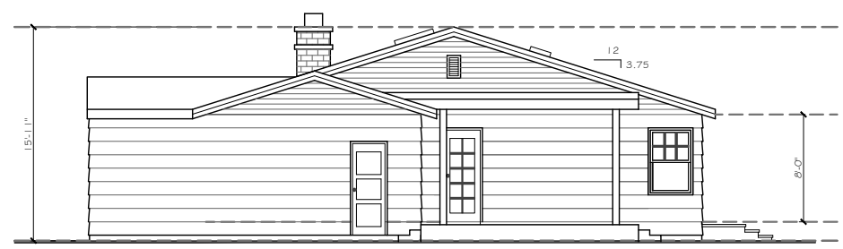
Existing East Elevation 1/4" = 1'-0"
