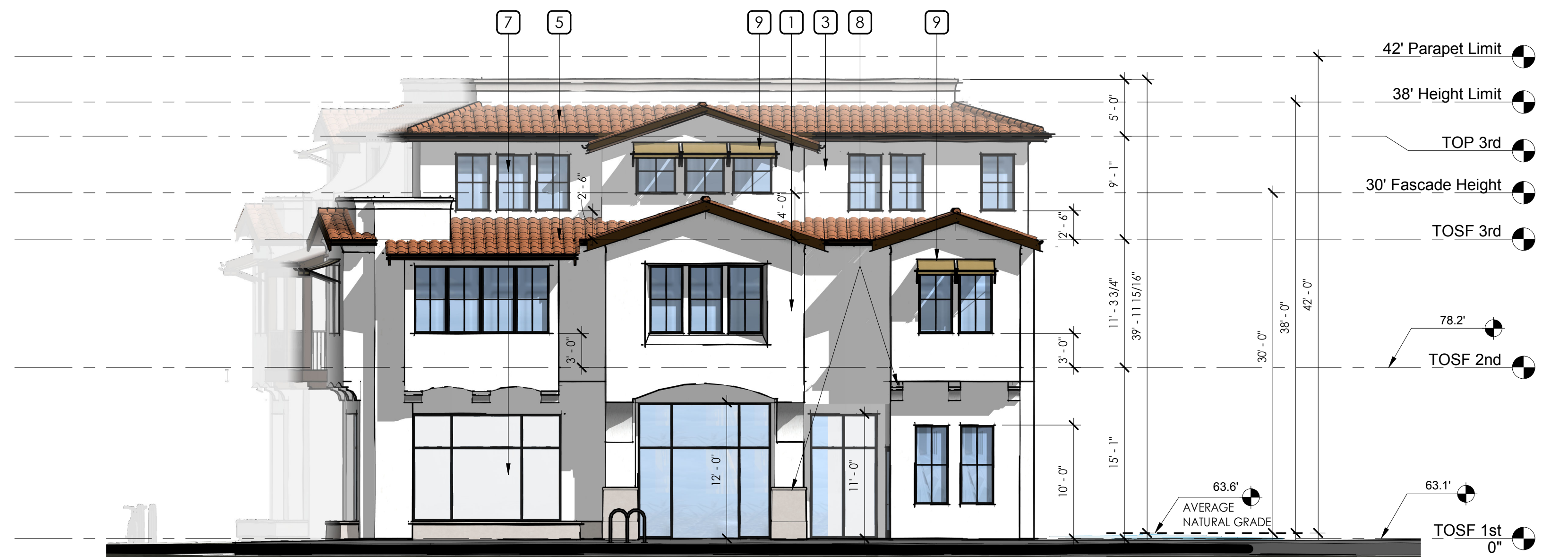
2 MIXED USE - NorthEast Elevation (El Camino Real) 1/8" = 1'-0"
