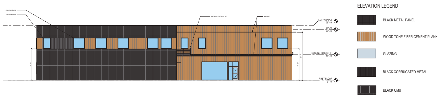
BLDG B - EXTERIOR ELEVATION NORTH 1/8" = 1'-0" 1
