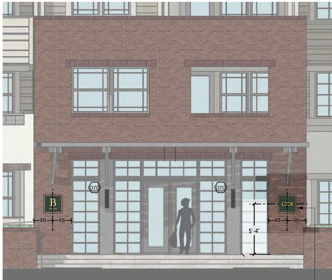
BUILDING B LOBBY ENTRY CONTEXT ELEVATION Scale: 3/16" = 1'-0"
