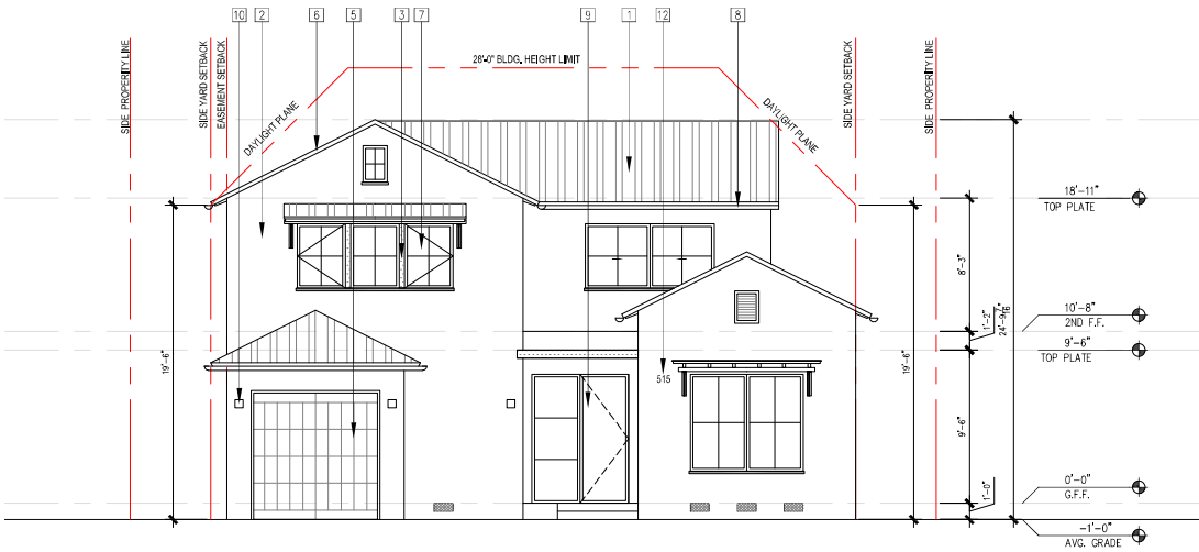
PROPOSED FRONT ELEVATION 01 Scale: 1/4"=1'-0"
