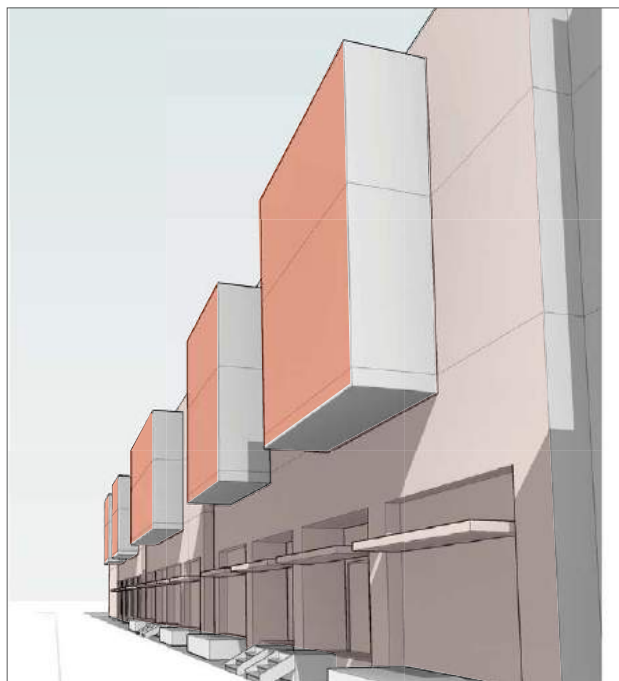
Figure E8. Allowable Building Projection Area
