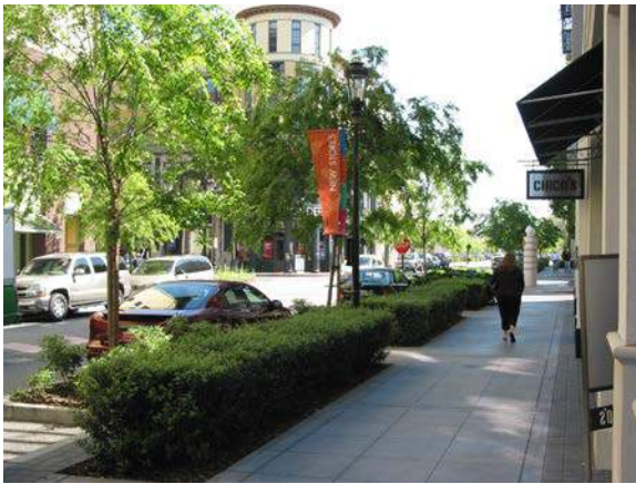
Sidewalk with clear zone and planting zone (Santa Cruz, California)
