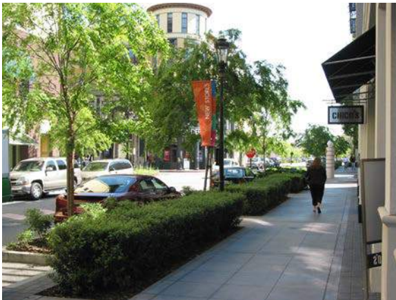
Sidewalk with clear zone and planting zone (Santa Cruz, California)
